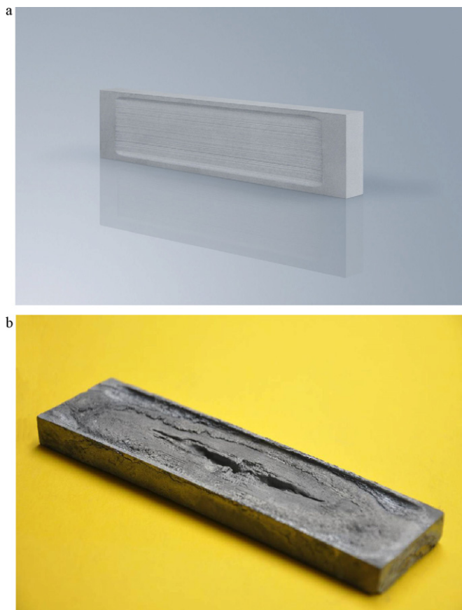
Fig. 1. Typical evaporation boat (a) and photo of an evaporation boat after application (b). The remaining metal is clearly visible.
